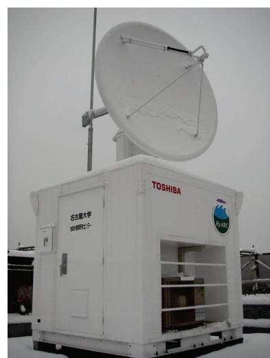
A new X-band polarimetric Doppler radar situated at Nagoya University.
